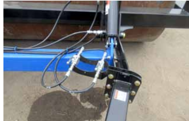
Shut-Off Valves (Float)
